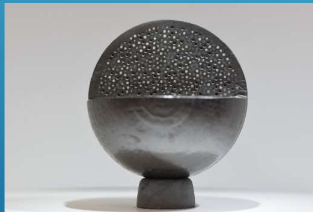
TRISO Fuel Pebble Cutaway
