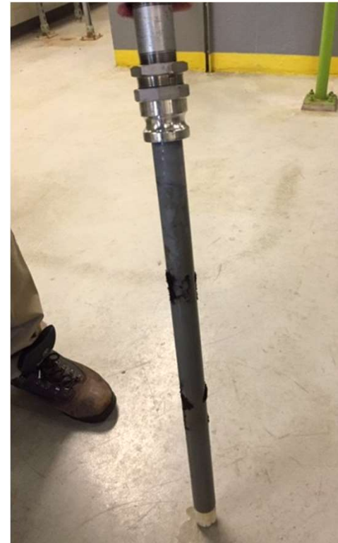
Magnetic rod removed for cleaning
