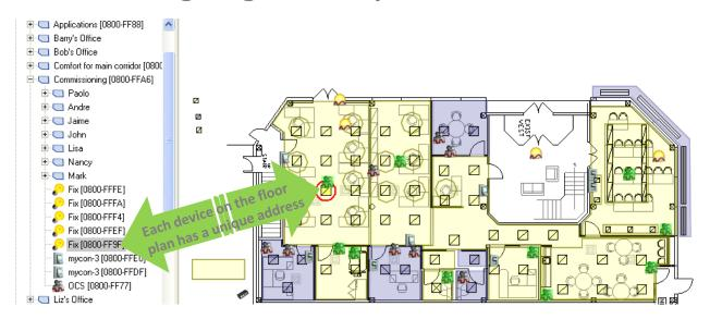
□ Once installed commissioning and administration of the entire system can be performed via the front-end software.
